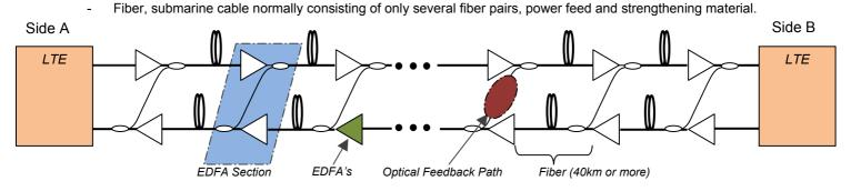
Fig 1; Major components of a Submarine System
