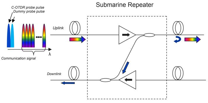
Fig 2; Submarine Repeater system showing C-OTDR return path.
